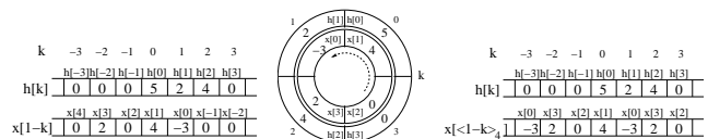
Figure 76: Problem 52: Convolution depicted with "flip and slide" method, (a) left, linear convolution, (b) right, circular convolution with N = 4 . As an example, in both cases the convolution sum is computed at n = 1 .
