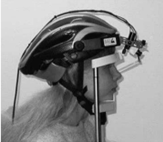
Figure 1: The head-mounted eye tracker device
