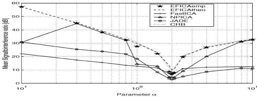
Figure 3.2: The Mean Signal-to Inference Ratio of EFICA, compared to CRB and some other ICA algorithms
