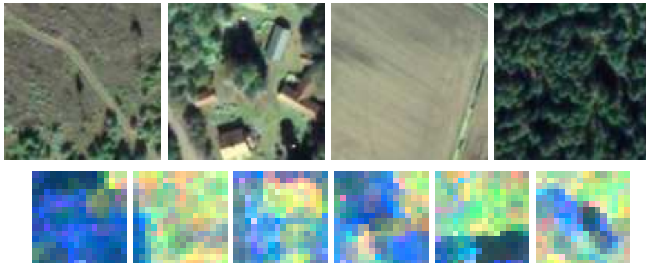
Figure 7.3: 100 \times 100 -pixel optical and 16 \times 16 -pixel SAR (Pauli decomposition) imagelets.
