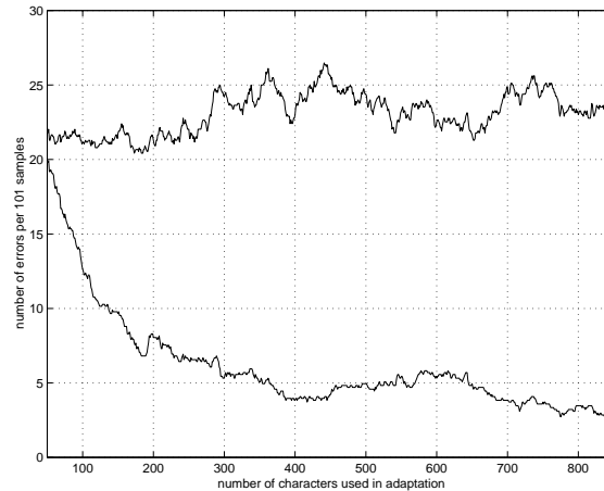
Figure 91: Evolution of the error rate during data collection in which the characters were recognized on-line. In the true data collection corresponding to the lower plot, input characters were added to the prototype set if one of the four nearest prototypes belonged to wrong class. The higher plot illustrates the nonadaptive simulation of the data collection. These result are obtained by averaging the result of eight writers.
